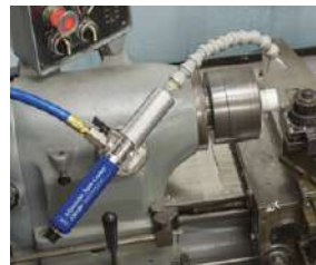
The Adjustable Spot Cooler maintains critical tolerances on machined plastic parts.
