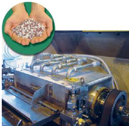
(4) Model 3250 Vortex Tubes cool the cutting knives in this pelletizer to prevent irregular shapes.
