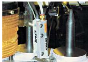
A Model 7103 3" (76mm) Standard Ion Air Knife removes dust from computer hard disks prior to assembly.
