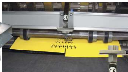
The Ionizing Point can be machine or duct mounted.
