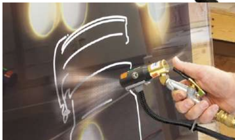
The Model 8293 Ion Air Gun cleaning artwork and glass prior to framing.
