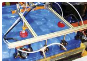
Model 8192 Ion Air Cannons provide static elimination in between solar panel lenses to assist separation of the lenses during production.
