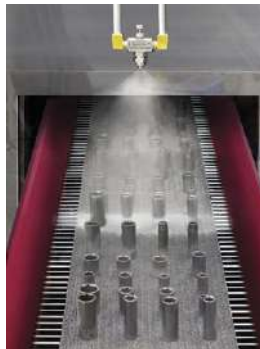
A Model SF1020SS is used to apply a light coating of oil to prevent sockets from rusting prior to a packaging operation.
