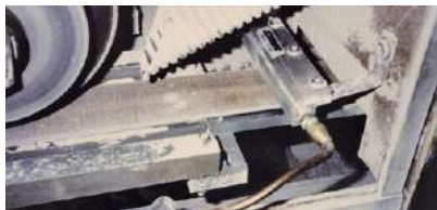
A Model 2006 6" (152mm) Standard Air Knife blows powder loose from a belt so it can be vacuumed away.
