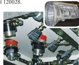
Model 120022 2" (51mm) Super Air Amplifiers and Model 1122 2" Flat Super Air Nozzles blow off transmissions after they are machined.
